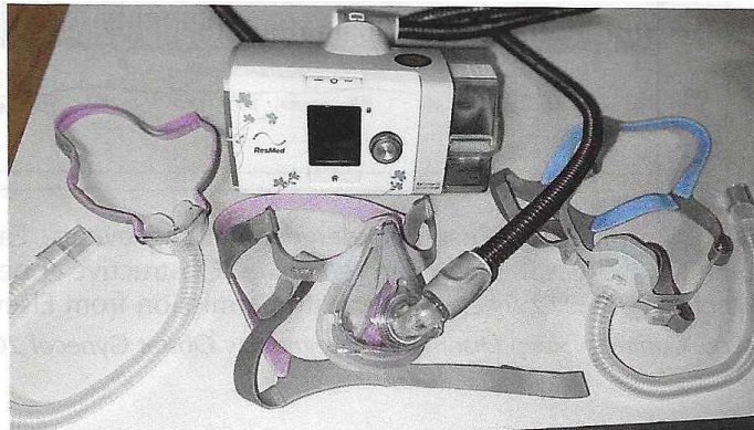
Figure 2. Continuous positive airway pressure (CPAP) machine and common masks. From left to right: nasal pillows, full face mask, and nasal mask.
